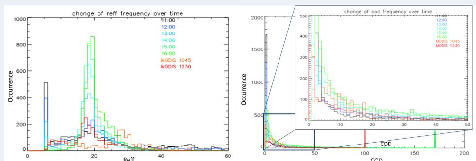
Figure 2: Histogram of Reff (left) and COD (right) in a scene over western Germany from 05/23/2012. The lines in black, blue and green show data from different images of SEVIRI and for comparisons MODIS data are included in red and orange.
