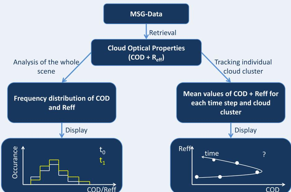
Figure 1: Schematic structure of the method used to analyze the development of optical cloud properties during the life-cycle of convective cells.
